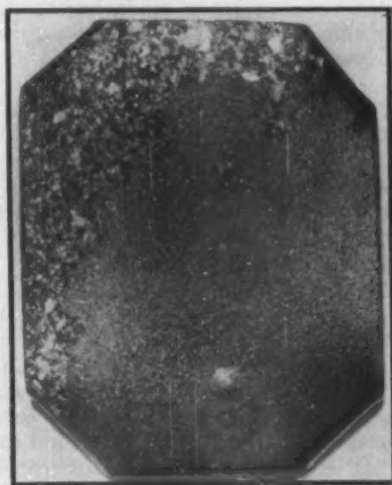
FIG. 1. An example of a large single crystal in a \text{Cu}_2\text{O} plate obtained by oxidizing a 1-in. \times \frac{1}{4} -in. \times 0.010 -in. Cu plate for 1 hr. at 1050^\circ\text{C} and annealing for 5 hr at 1100^\circ\text{C} .
